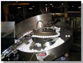
The DTM/CapTech centrifugal cap feeder was specifically designed to be extremely flexible and capable of sorting and feeding a wide range of cap shapes and sizes including irregular shapes.
