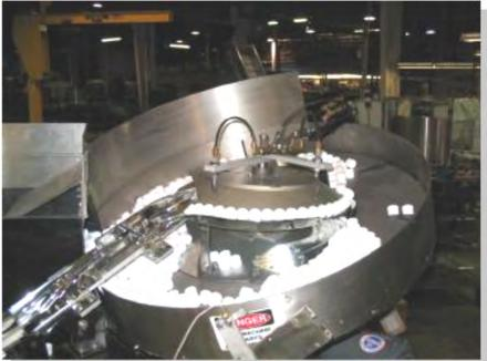
The centrifugal cap feeder was specifically designed to be extremely flexibility and capable of sorting and feeding a wide range of cap shapes and sizes including irregular shapes.
