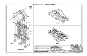
The difficult and high-risk areas of the design are modeled or prototyped to assure success and steady progress in completing the task. Once a concept is clarified, an overall design layout is created. After design reviews, detailed drawings are produced for parts fabrication.
